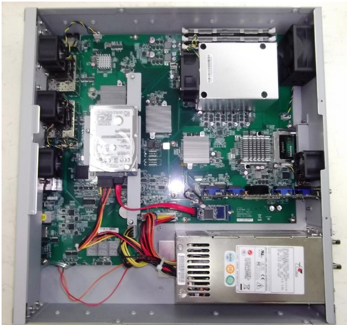
Internal view of unit with dual AC power supply
