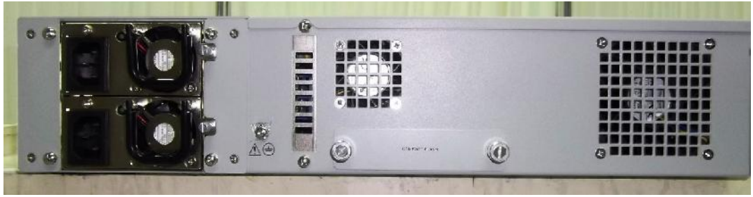
Rear side of unit with dual AC power supply
