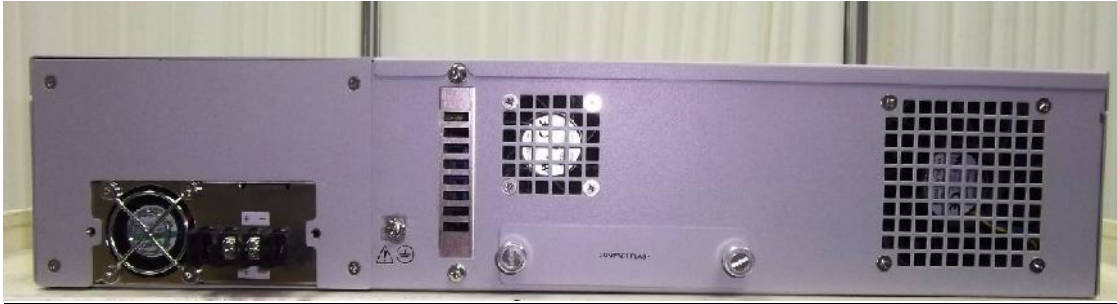
Rear side of unit with single DC power supply
