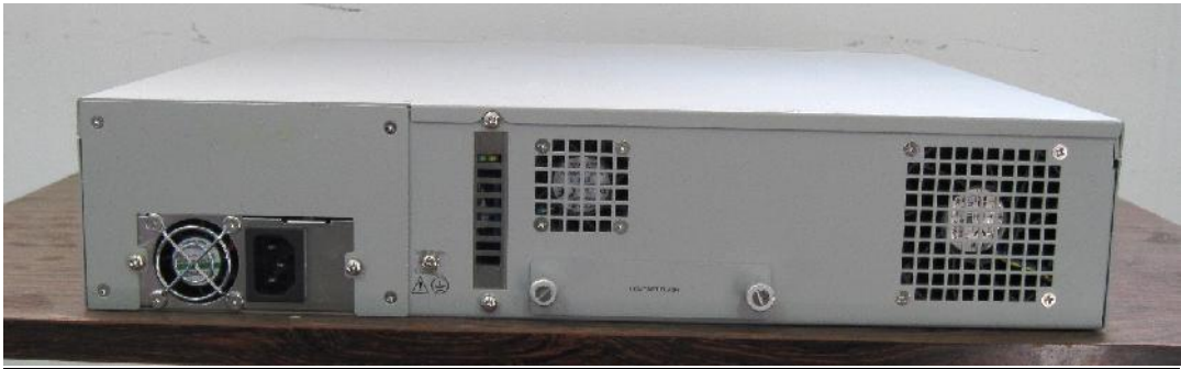
Rear side of unit with single AC power supply
