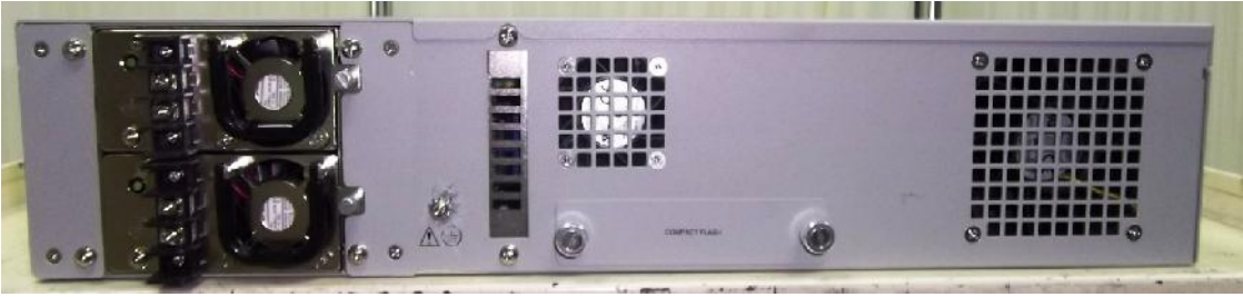
Rear side of unit with dual DC power supply
