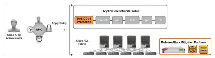
Figure 1: Radware Attack Mitigation System (AMS) and Cisco ACI
