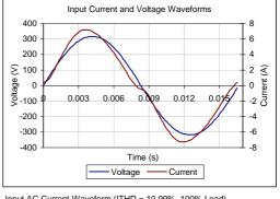
Input AC Current Waveform (ITHD = 10.99%, 100% Load)
