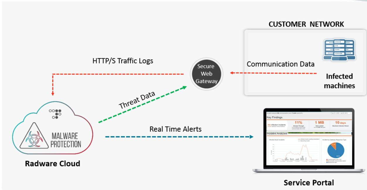
Figure 7: Diagram of solution architecture that outlines how Radware identified the malware bypassing the Secure Web Gateway
