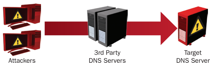
Figure 13: In a Reflective DNS attack an attacker sends DNS requests to third-party servers, while spoofing the source IP of the request to be that of the target server (the victim). The reply sent by third-party servers is sent to the target DNS server, amplified 3-10x times.
