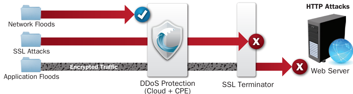
Figure 18: HTTPS-based attacks are not detected by cloud or CPE device mitigation solutions. An application-level HTTPS attack is encrypted and cannot be analyzed by the mitigation gear. In addition, HTTPS is vulnerable to unique SSL Attacks.
