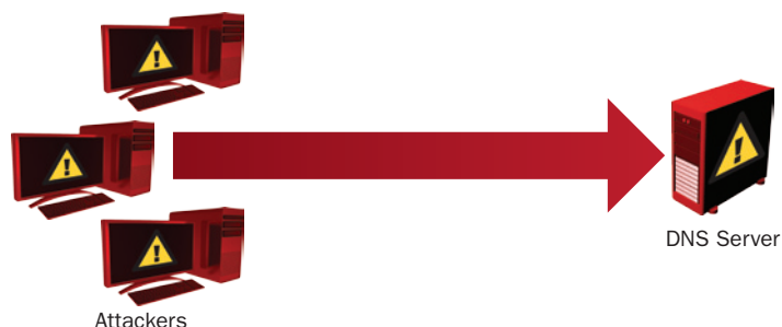
Figure 12: In a Basic DNS flood , an attacker sends numerous DNS requests to the target DNS Server, flooding the server with requests and bringing it down.
