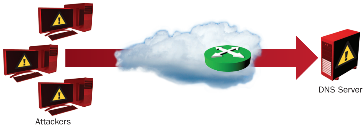
Figure 16: In a Garbage DNS flood , the attacker floods the DNS server with large data packets sent to its UDP port 53. This attack exploits the fact that organizations will always leave the DNS port open and will not block traffic at the router level.
